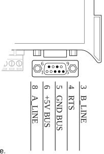
For connection to the Profibus Master, use a standard Profibus cable.
