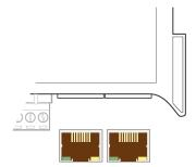
To connect to the MASTER, use a standard twisted pair Ethernet cable with RJ45 connector.
